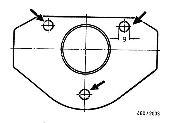
3 hexagon bolts M 8  $\times$  40 mm are to be used to clamp pumps with slots to the pump flange.
